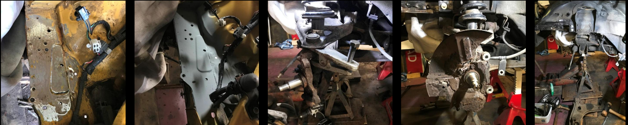
Photo below: The front near-side top & bottom wishbones and suspension leg removed ready for reconditioning and upgrade.
