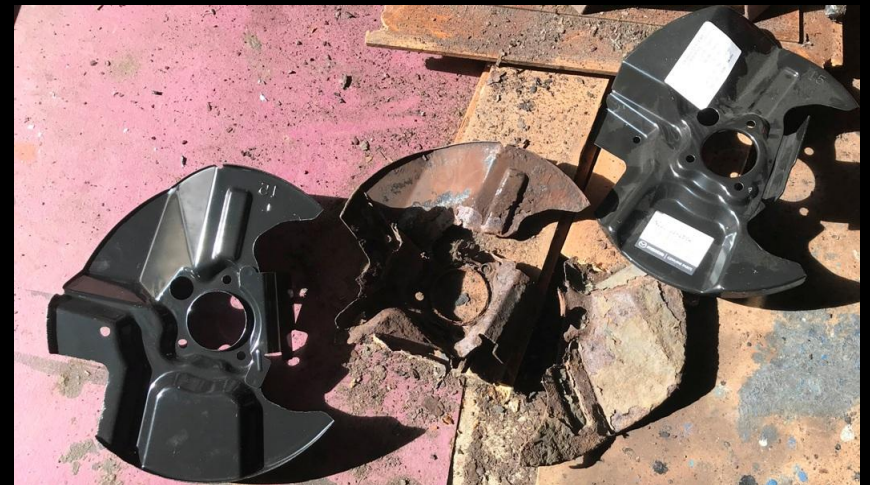
Photo below: Shows the old rusty front disc back-plates (totally corroded) situated between the two new shiny Mazda supplied brake back-plates (seen here on either side of the rusty remains).
