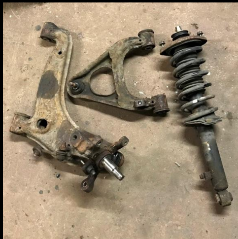
Photo below: The front near-side top & bottom wishbones and suspension leg removed ready for reconditioning and upgrade.
