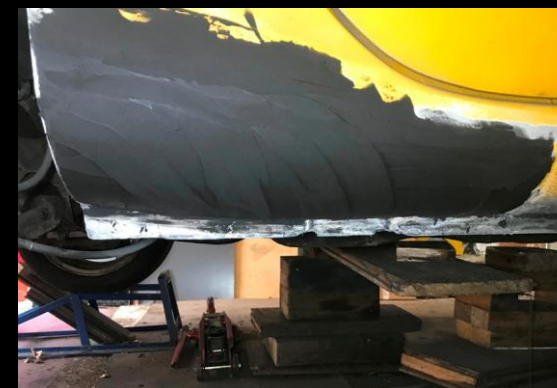
Once fully welded; all seams Tiger Sealed
