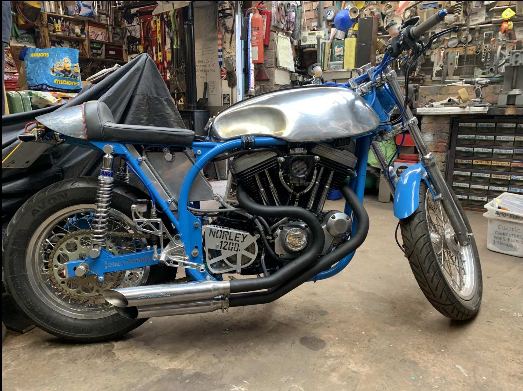
With my new-look exhaust pipes . . . Painted using VHT Black oil & petrol resistant paint (protects up to 800° C) 28 th May 2023
