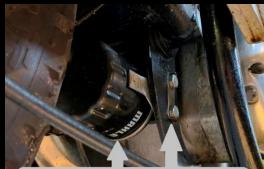
This is missing on my Commando, so this will be one of the 1st modifications that I make - a remote, spin-off oil filter added to the underside sub-frame.
