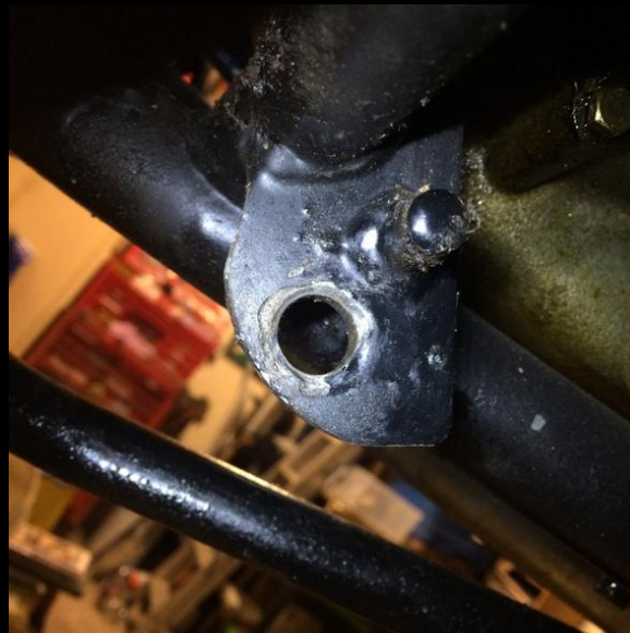
I re-bushed the Central Stand pivot points and this proved effective, taking all of the 'play' out of the Stand. Central Stand refitted – job done!
