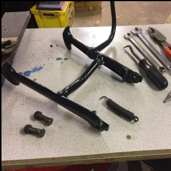
I re-bushed the Central Stand pivot points and this proved effective, taking all of the 'play' out of the Stand. Central Stand refitted – job done!
