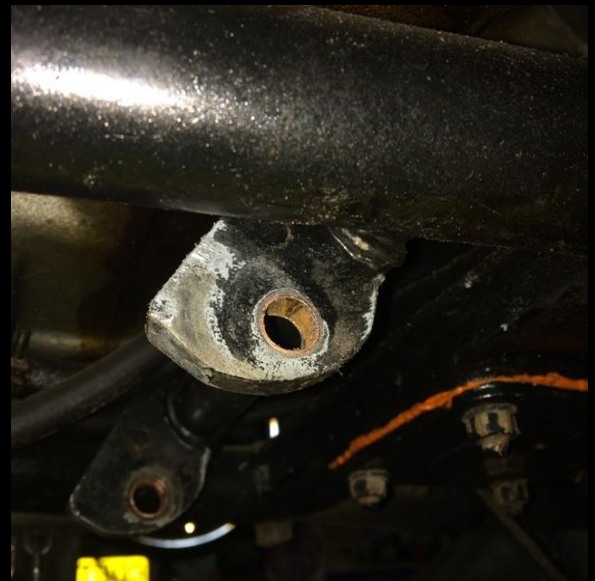
I re-bushed the Central Stand pivot points and this proved effective, taking all of the 'play' out of the Stand. Central Stand refitted – job done!
