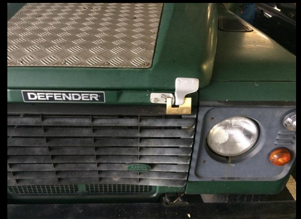
New FBLS fitted (above right photo). With Industrial Shutter type Pad Lock fitted for extra bonnet security.
