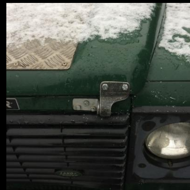
New FBLS fitted (above right photo). With Industrial Shutter type Pad Lock fitted for extra bonnet security.
