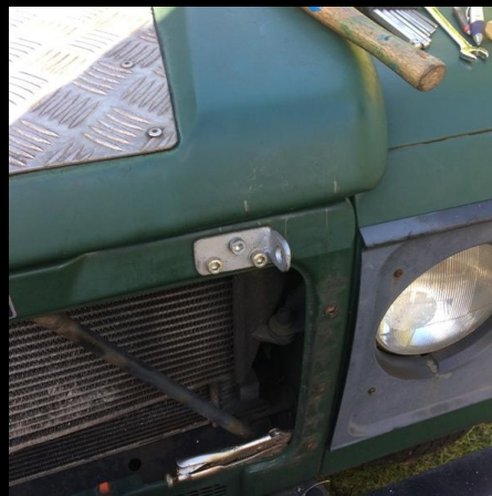
New FBLS fitted (above right photo). With Industrial Shutter type Pad Lock fitted for extra bonnet security.
