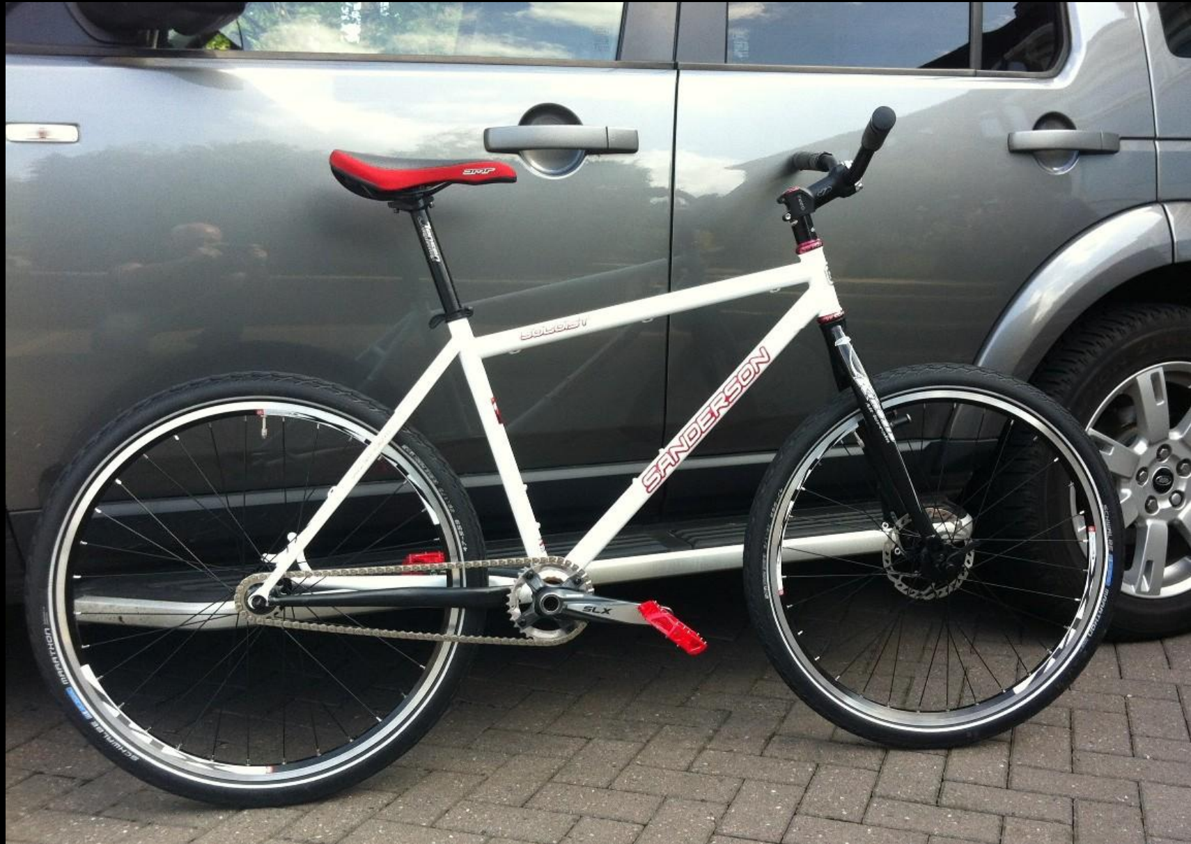
Sanderson 18" EBB Soloist Frame with VP Head Set, VP Bottom Bracket, Jenson Seat Post & DMR Race Saddle, Xero 90mm Riser, Independent Handlebars, Velo Lock-on Grips, Sanderson ProMag SL Pedals, Independent Seat Collar, Hope Head Spacers, Kinesis Forks, Shimano SLX Crank Set, 32T Front Chain-Ring, 16T Rear Sprocket, YBM BMX Half-Link Chain, 26" Wilkinson Wheels (on Shimano Hubs), Schwalbe Marathon Reflex Tyres, Shimano Disc Brake Rotor (but, No brakes fitted at this stage).
