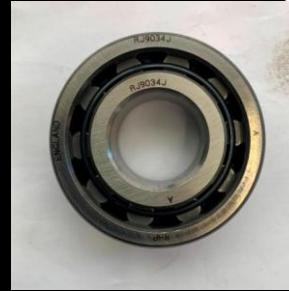
New Roller Main Bearing to be fitted.
