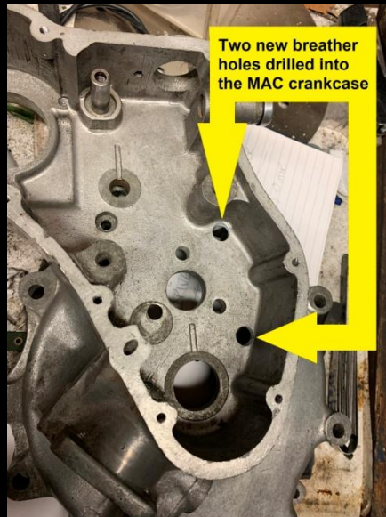
Two new breather holes drilled into the MAC crankcase to relieve c/c pressure.
