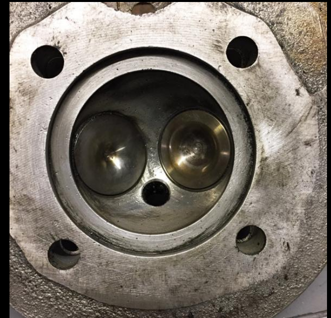
Photo above (right) shows the partly cleaned-up and partly de-coked cylinder chamber & valves.
