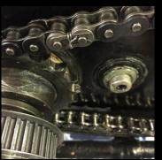
2<sup>nd</sup> Photo (left) is my method of bringing the primary chain 'together', in order to engage the chain 'Split Link' (the use of Lock Wire). And obviously (3<sup>rd</sup> photo left) I also 'Lock-Wire' the split link together.
