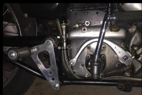
After fitting the new Rear-Set Footrests and gear change mechanism, I took the MAC out for a good test ride.
