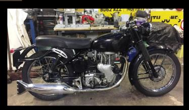
31<sup>st</sup> August 2020: I've finally got around to finishing-off the end of each footrest with an aluminium-turned-boss. Each one is now held in place by a stainless steel cap head bolt (countersunk into the aluminium boss), including the new (amended / redesigned) gear change lever. I decided to make three 'Fixed' footrests (rather than the usual 'Folding Footrests'). The only folding footrest now is on the front off-side (to clear the Kickstart Lever).
