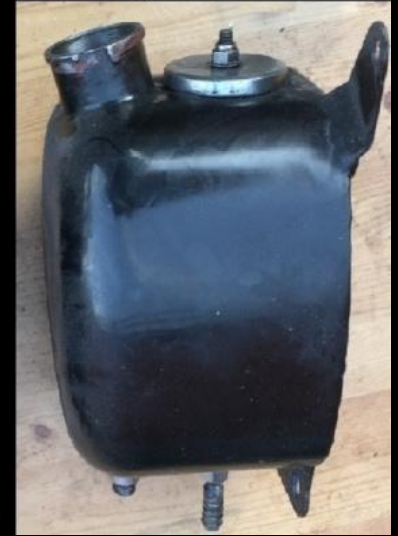
& MAC Oil Tank with longer Oil Filler Neck
