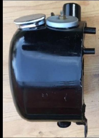
Venom Oil Tank with top hat Anti-Froth Breather
