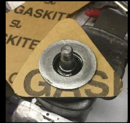
Zero Degrees in my Garage most mornings; hence the Big Winter Coat & Woolley Hat. BBbbbbrrrrrr! But, it's getting there, slowly but surely. The three photos down the right column show my home-made Gasket. The Gasket Paper was supplied by Velo Spares Ltd.
