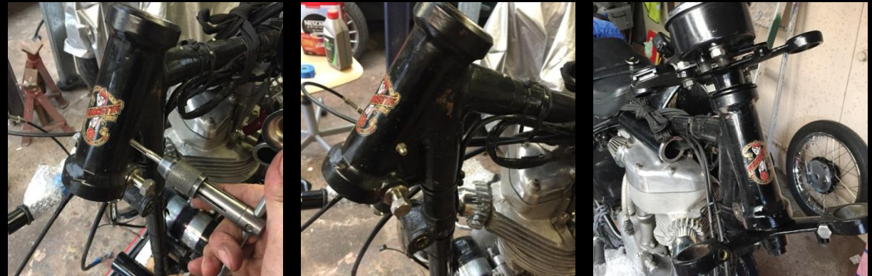
(Above photos) This Grease Nipple modification aids essential and regular grease maintenance
