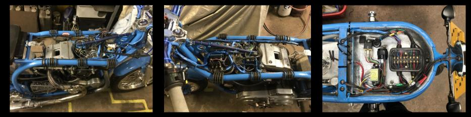
All of the electrical connectors and fittings have been 'crimped-on' & then soldered-on for good measure. I've used see-through insulating sleeves on all of the electrical connectors and tried to keep all the *electricals* neat & tidy. My Lithium Ion Battery (incredibly light-weight) is still going strong after 7 years.
