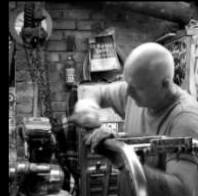
Photos Above & Below : Frame being polished in preparation for Powder Coating.
