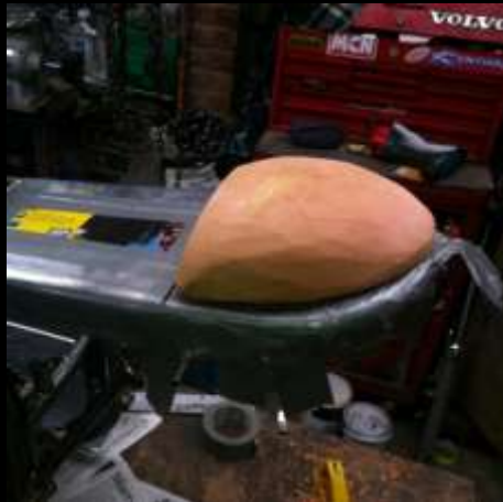
Seat No.2 being made. . . . (above photos) the next stage - after smoothing down & reshaping - is to 'lay-up' with Fibre Glass to make yet another mould.
