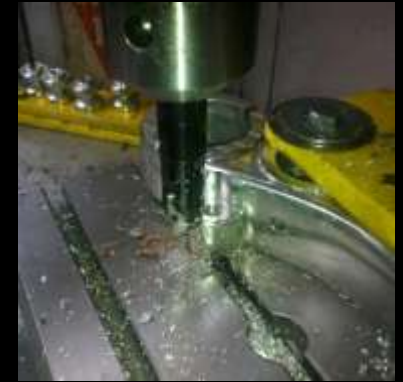
The Photos (above & below) show more milling, drilling and thread tapping to the Steering Yoke and other components. Plus, Cutting & Milling-out new Rear-Set Foot Rest plates.
