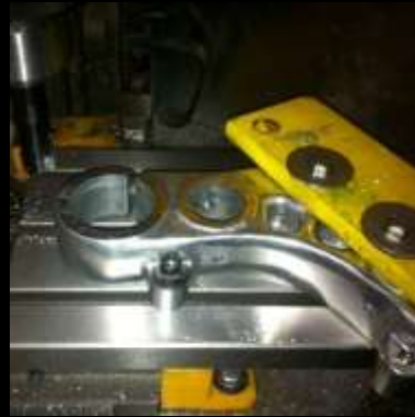
The Photos (above & below) show more milling, drilling and thread tapping to the Steering Yoke and other components. Plus, Cutting & Milling-out new Rear-Set Foot Rest plates.
