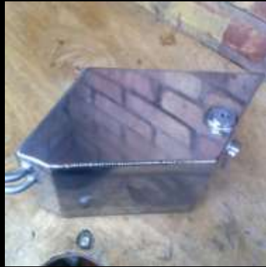
The Oil Tank before polishing & after the first polish (stage one)! The rear mudguard plate in position & the Perspex template for the rear brake calliper
