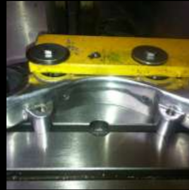
The Photos (above & below) show more milling, drilling and thread tapping to the Steering Yoke and other components. Plus, Cutting & Milling-out new Rear-Set Foot Rest plates.
