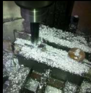
The Photos (above & below) show more milling, drilling and thread tapping to the Steering Yoke and other components. Plus, Cutting & Milling-out new Rear-Set Foot Rest plates.
