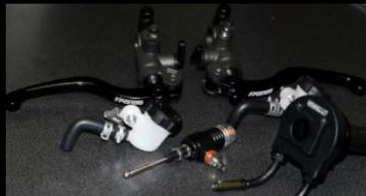
Frando Hydraulic Brake & Clutch Master Cylinders ( Handlebar Levers) & Hydraulic Slave Cylinder for the Clutch (below), with Venhill Quick-action
