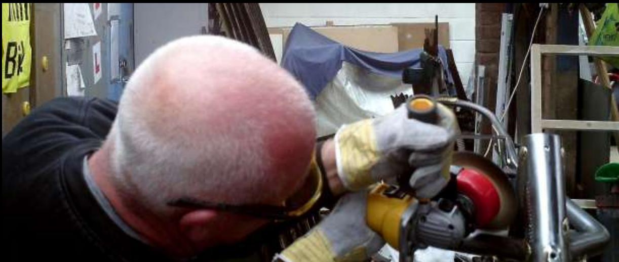
Photos Above & Below : Frame being polished in preparation for Powder Coating.
