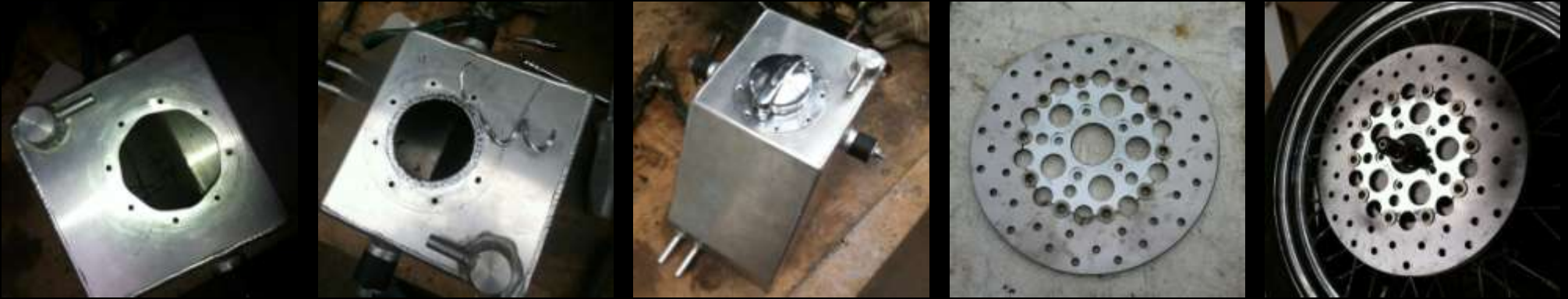
(Photo above) New Front & Rear 'Floating' Disk Brake Rotors.
