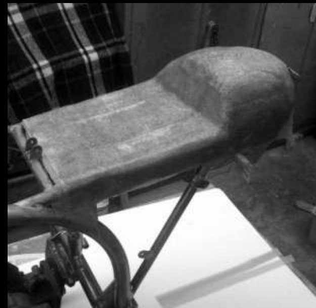
Seat No.2 being made. . . . (above photos) the next stage - after smoothing down & reshaping - is to 'lay-up' with Fibre Glass to make yet another mould.
