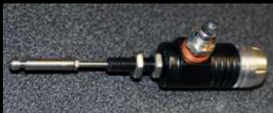
Frando Hydraulic Brake & Clutch Master Cylinders ( Handlebar Levers) & Hydraulic Slave Cylinder for the Clutch (below), with Venhill Quick-action
