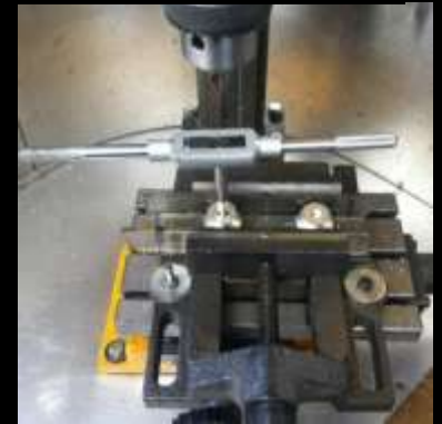
The Photos (above & below) show more milling, drilling and thread tapping to the Steering Yoke and other components. Plus, Cutting & Milling-out new Rear-Set Foot Rest plates.
