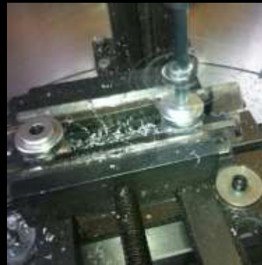
The Photos (above & below) show more milling, drilling and thread tapping to the Steering Yoke and other components. Plus, Cutting & Milling-out new Rear-Set Foot Rest plates.
