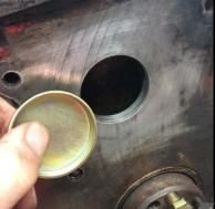
The 'First Job' was to remove the engine from the car to fix the water leak. No real surprise, as the 'Car for Sale Advert' stated; "this car needs the rear core plug fixing, it's quite difficult to reach so this will be a job for the new owner". So! That'll be me then !!!
