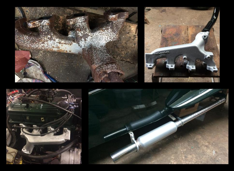
No expense was spared as two brand new 'U' Clamps were fitted, plus new heat-shield wrap & high-temperature 'silver' paint applied to the Silencer. Job Done !
