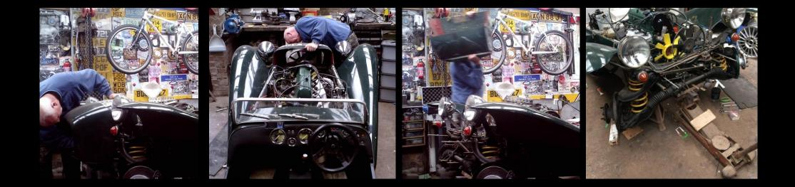
The Nose Cone was removed for some Fibre Glass repairs (above). And ... I've hand-made two Fibre Glass Covers (photos below): One to fit over the exposed Steering Column and a second one to fit over the Clutch & Brake Pedal Housing. The original covers (for both column & pedal housing was made of sheet aluminium - 'folded' into a rudimentary 'box' shape). I think this new design occupies the space better and looks less of a 'bodge' and more of a thought-out purpose-built approach.
