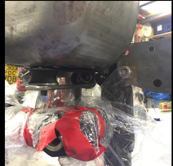
The photos below: show a close-up of the newly fabricated Oil Tank Bracket (Rubber Mounting), made to hold & isolate the Oil Tank from any Frame vibrations. It's quite a sturdy bracket as it has to take the weight of a full tank of engine oil. That's why I have used the same type of Rubber Mounting Spool
