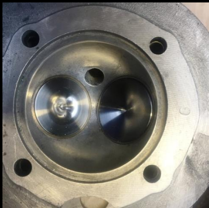
New Valves & Helicoil fitted to the Spark Plug thread and New Amal 389/15 Carburetter & Filter purchased in readiness for the rebuild (photos below).
