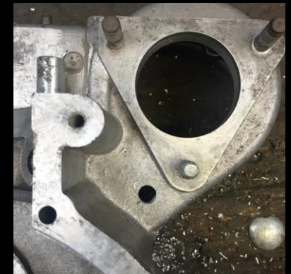
Photos below: To make sure 'Drilling & Tapping' is 'Square', I used my little Mill / Drill.
