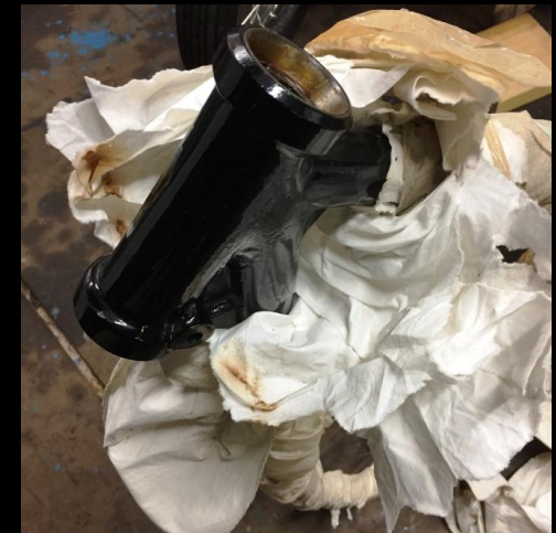
The two photos below: Reconditioned & repainted Frame wrapped-up ready for the 'Re-Build'. New Trunnion Shaft & Bushes plus Frame re-alignment carried-out by Ralph Seymour's.
