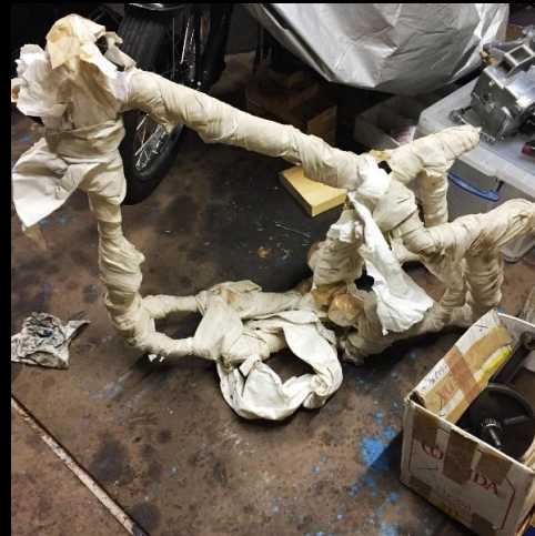
The two photos below: Reconditioned & repainted Frame wrapped-up ready for the 'Re-Build'. New Trunnion Shaft & Bushes plus Frame re-alignment carried-out by Ralph Seymour's.
