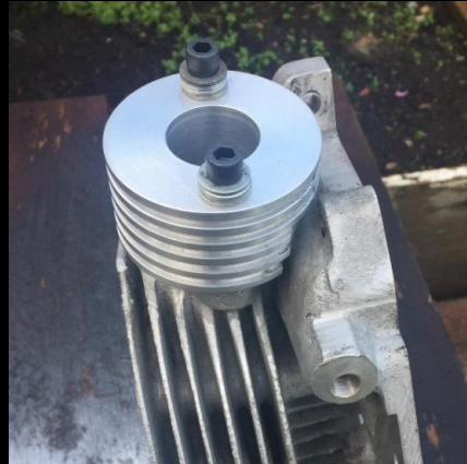
New Valves & Helicoil fitted to the Spark Plug thread and New Amal 389/15 Carburetter & Filter purchased in readiness for the rebuild (photos below).
