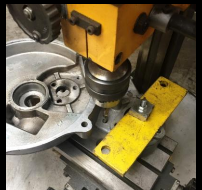
Photos below: To make sure 'Drilling & Tapping' is 'Square', I used my little Mill / Drill.
