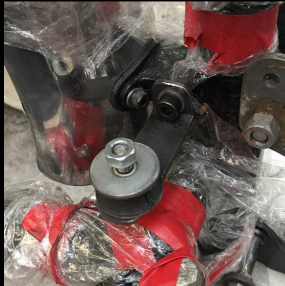
The photos below: show a close-up of the newly fabricated Oil Tank Bracket (Rubber Mounting), made to hold & isolate the Oil Tank from any Frame vibrations. It's quite a sturdy bracket as it has to take the weight of a full tank of engine oil. That's why I have used the same type of Rubber Mounting Spool
