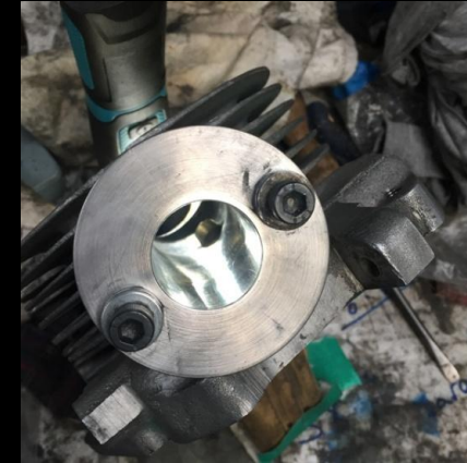
New Valves & Helicoil fitted to the Spark Plug thread and New Amal 389/15 Carburetter & Filter purchased in readiness for the rebuild (photos below).
