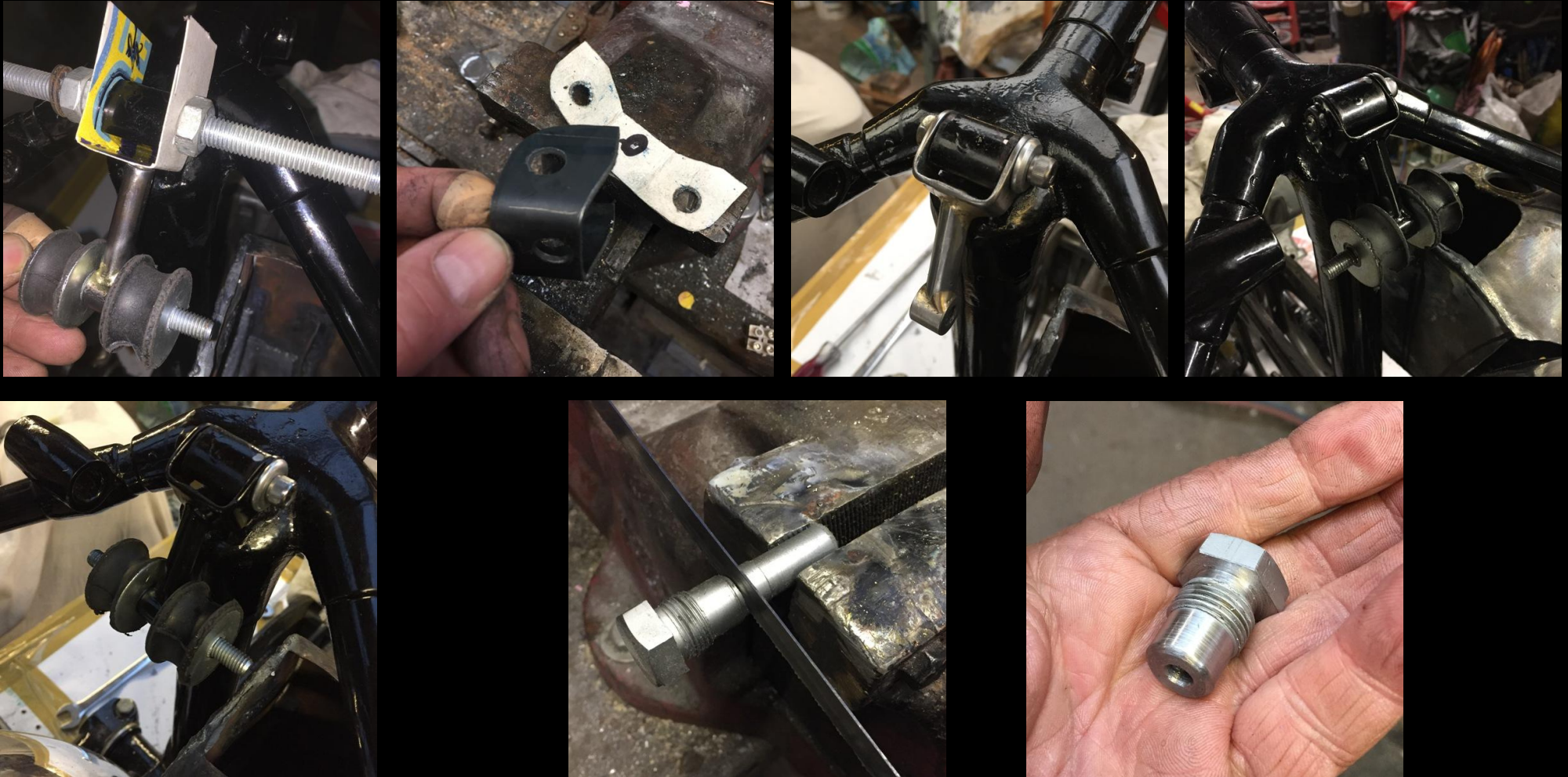
Above photos show the Oil Suction Plug being Sawn down, just like I did for the MAC.
