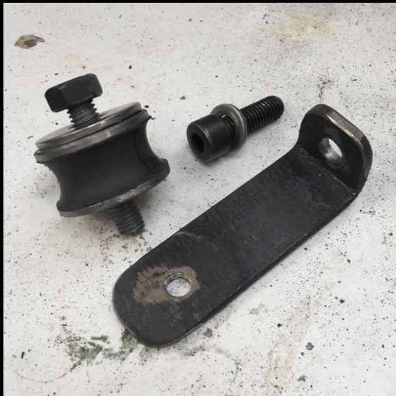
The photos below: show a close-up of the newly fabricated Oil Tank Bracket (Rubber Mounting), made to hold & isolate the Oil Tank from any Frame vibrations. It's quite a sturdy bracket as it has to take the weight of a full tank of engine oil. That's why I have used the same type of Rubber Mounting Spool
