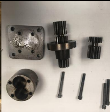
(Photos below) Pushrods & Inner Clutch Housing Plate cleaned-up on the Myford Lathe and I've dismantled the Oil Pump for inspection
