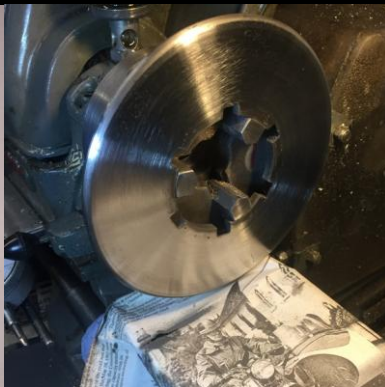
(Photos below) Pushrods & Inner Clutch Housing Plate cleaned-up on the Myford Lathe and I've dismantled the Oil Pump for inspection
