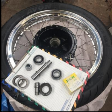
New Wheel bearings fitted to both wheels.
