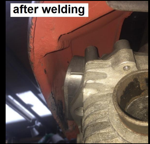
The photo (above right) shows the clearance gained by 'recessing' the Tank.
