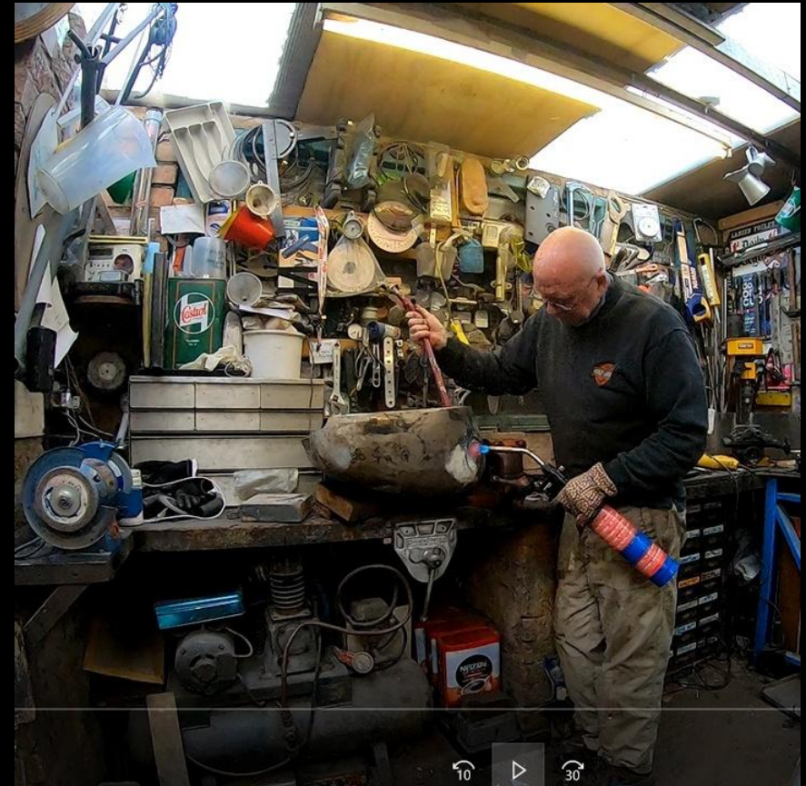
Cylinder Studs (1 st two photos below left = before & after cleaning), plus Crankcase Stud 'Threads' being cleaned-up and re-tapped (3/8" BSF thread).
