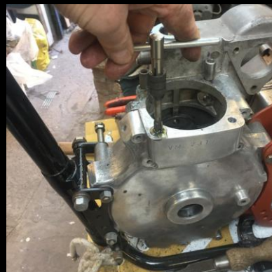
Cylinder Studs (1 st two photos below left = before & after cleaning), plus Crankcase Stud 'Threads' being cleaned-up and re-tapped (3/8" BSF thread).
