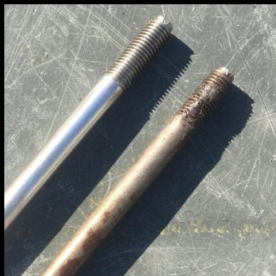
Cylinder Studs (1 st two photos below left = before & after cleaning), plus Crankcase Stud 'Threads' being cleaned-up and re-tapped (3/8" BSF thread).
